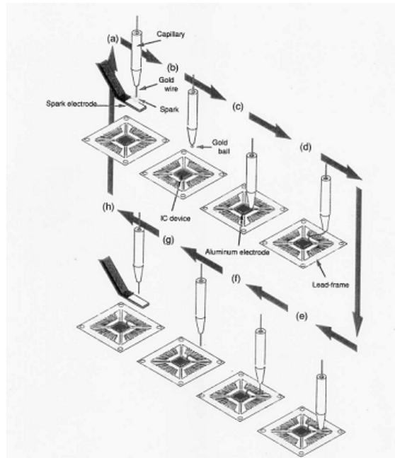
Fig.1 – Wire bonding process
