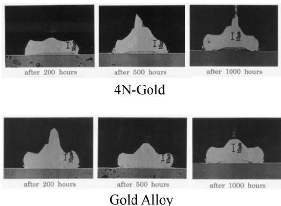
Fig.4 – Cross-section observations of temperature storage samples
