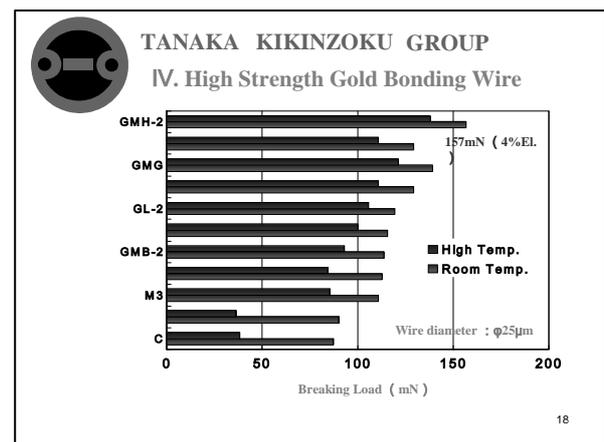
High strength methods are types, volume and mixing of elements. General gold bonding wire keeps 4N-purity. This drastic change of property by less than 100 wtpm elements is based on field results in high purity metal research.
