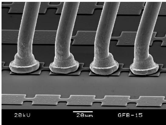
Fig.2 – Fine pitch bonding
