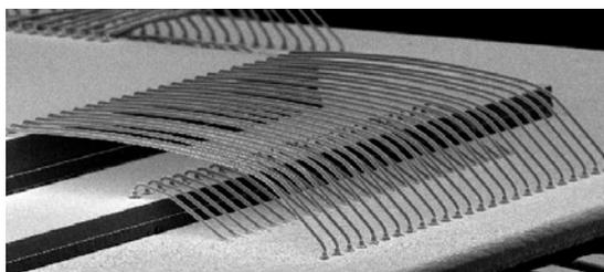
Fig.3 – Stacked bonding
