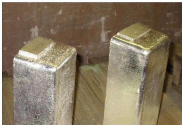
silver bars cast in a closed mould will have a sprue on one end. This is part of the gating system that feeds molten silver into the mould cavity. The sprue is normally guillotined off, producing a relief at the end of the bar, which can have sharp edges, making the bars dangerous to handle.
